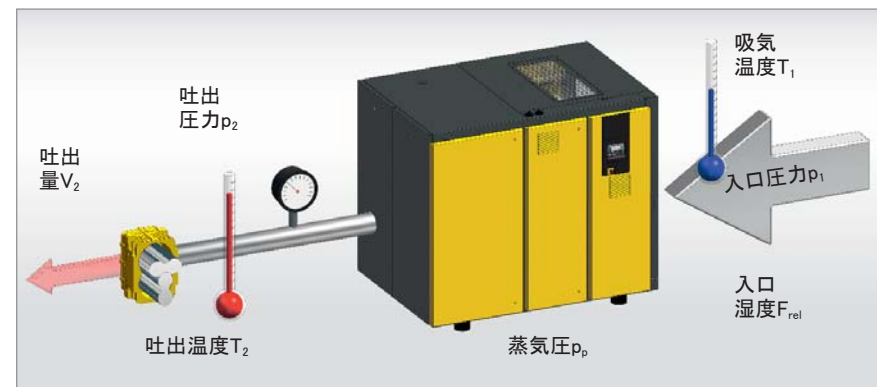
図1: 吐出空気量の測定 (ISO 1217, Appendix C (DIN 1945, Appendix F))
